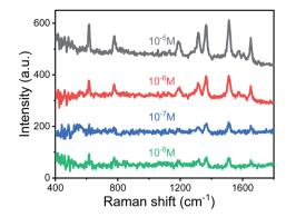
Fig. 7 Raman spectra of R6G with concentrations ranging from  $10^{-5}~\mathrm{M}$  to  $10^{-8}~\mathrm{M}$  detected by a portable Raman spectrometer. The output light from the Raman probe head was coupled into a multimode fiber which aligns with the capillary using a common flange optical fiber connector.
