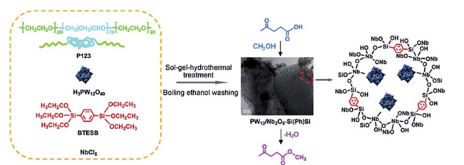
Fig. 8 Preparation route for phenylene-bridged 2D ordered mesoporous PW 12 /Nb 2 O 5 -Si(Ph)Si and the catalytic reaction. 84 Reproduced with permission. 84 Copyright 2016, Elsevier.
