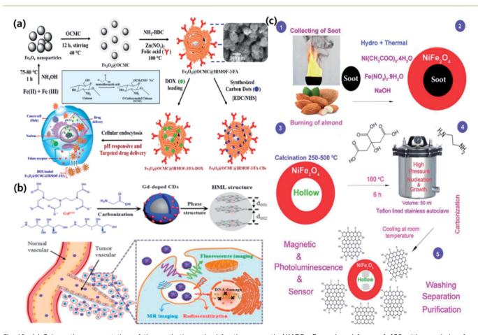
Fig. 10 (a) Schematic representation of the synthetic method for the magnetic NMOFs. Reproduced from ref. 126 with permission from American Chemical Society, copyright 2016. (b) Synthesis approach of Gd-doped C-dots by hydrothermal treatment of GDPA and glycine and following applications. Reproduced from ref. 127 with permission from Elsevier, copyright 2017. (c) Preparation of C-dot and hollow magnetic nanocomposite. Reproduced from ref. 129 with permission from Elsevier, copyright 2019.
