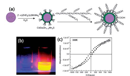
Fig. 2 (a) Synthesis procedure for the fabrication of water soluble core/shell CdSe/ $Zn_{1-x}Mn_xS$ . Reproduced from ref. 65 with permission from American Chemical Society, copyright 2007. (b) Fluorescence of yellow-emitting QDs (right) and DI water (left) under 366 nm UV source and (c) magnetization curve for QDs. Reproduced from ref. 70 with permission from American Chemical Society, copyright 2005.
