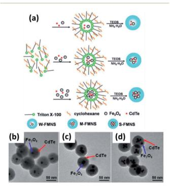
Fig. 5 (a) Schematic of the preparation of (CdTe/Fe<sub>3</sub>O<sub>4</sub>)@SiO<sub>2</sub> FMNS with various magnetic potentials via reverse microemulsion method. TEM images of (CdTe/Fe<sub>3</sub>O<sub>4</sub>)@SiO<sub>2</sub> FMNS: (b) W-FMNS, (c) M-FMNS, and (d) S-FMNS. Reproduced from ref. 99 with permission from American Chemical Society, copyright 2014.
