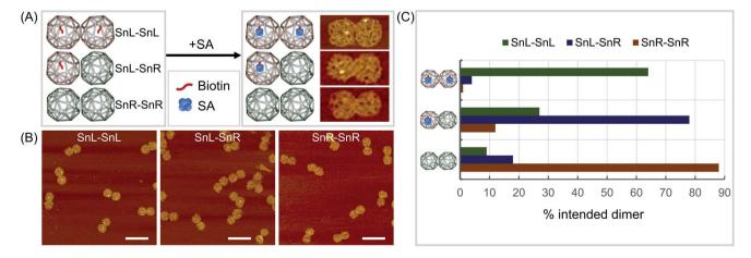
Fig. 3 Validation of chirality. (A) Schematic diagrams (left) and AFM results after reaction with biotin (right) showing the different produced Sn dimers, biotin modifications and SA attachment where SA is visible in AFM images as white dots. (B) Wider field AFM images of the 3 forms of Sn dimers after reaction with biotin for bound SA with dimer structures of SnL-SnL (left), SnL-SnR (middle) and SnR-SnR (right). (C) Quantitation of intended dimers formed. AFM scale bars represent 200 nm.
