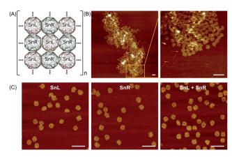
Fig. 5 2D arrays of Sn origami. (A) Schematic illustration of the array, (B) AFM images of the 2D structure (left) and a magnified image (right) and (C) AFM images of SnL (left) and SnR (middle) alone without staple modifications and after mixing together SnL + SnR (right), showing no interaction in absence of connecting staples. AFM scale bars represent 200 nm.
