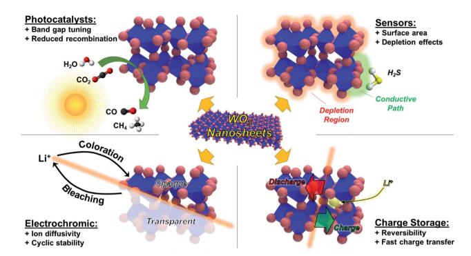
Fig. 1 Schematic showing basic principles of operation for WO<sub>3</sub> in photocatalysts, sensors, electrochromic devices, and charge storage applications, along with the potential advantages provided by the nanosheet morphology.
