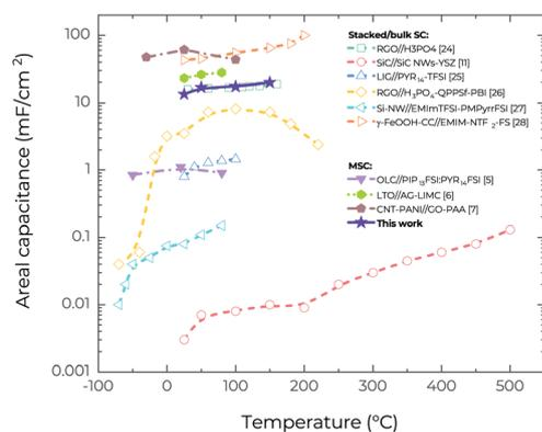
Fig. 5 Comparison of the areal capacitance of high-temperature supercapacitors in the literature to date, including both planar MSCs and stacked supercapacitors. Here, the areal capacitance for this work is in the voltage window of 1.0 V.
