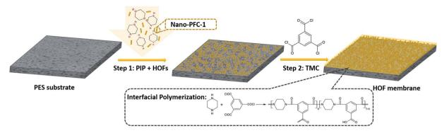
Scheme 1 The preparation process of a HOF-TFN membrane containing PFC-1 nanoparticles via interfacial polymerization.
