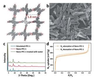
Fig. 1 (a) The two-dimensional porous structure of PFC-1. (b) A scanning electron microscopy (SEM) image, (c) powder XRD patterns, and (d) the N<sub>2</sub> adsorption/desorption isotherm (77 K) of Nano-PFC-1.
