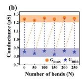
Fig. 6 Flexibility characteristic of the Al/PVP–NCQD/ITO synaptic device. (a) Pulse trains (50 positive and 50 negative pulses, 2 V, 10 ms) applied to the device after different bending numbers N. (b) Statistical values of  $G_{\text{max}}/G_{\text{min}}$  under different bending numbers.
