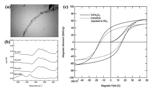
Fig. 3 (a) TEM images of  $CoFe_2O_4$  MNPs. (b) FTIR spectra of the native MNPs before exposure to sulfur dioxide as well as MNPs after exposure (test 1) and MNPs after exposure but without desorption (tests 2 and 3). (c) Magnetic susceptibility curves for MNPs both before and after sulfur dioxide breakthrough experiments. Reprinted with permission from ref. 33. Copyright (2012) American Chemical Society.
