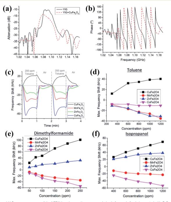
Fig. 13 (a and b) Frequency response of the MSSW-based magnetic gas sensor device before and after being coated with  $CuFe_2O_4$  nanoparticles. (c) Response of the magnetic gas sensors based on spinel oxides for 200 ppm toluene at room temperature. The response of the magnetic sensors at different concentrations of (d) toluene, (e) dimethylformamide, and (f) isopropanol. Reprinted with permission from ref. 84. Copyright (2017) Elsevier.
