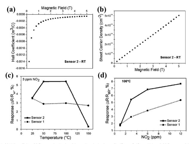
Fig. 6 (a) Hall coefficient. (b) Sheet carrier density of the as-deposited galinstan film (Sensor 2,  $10 \mu m$  thickness). (c) Response of the as-deposited sensors towards 3 ppm  $NO_2$  as the function of the operating temperature. (d) Response amplitude of the as-deposited sensors as a function of  $NO_2$  concentration. Reprinted with permission from ref. 48. Copyright (2017) Elsevier.
