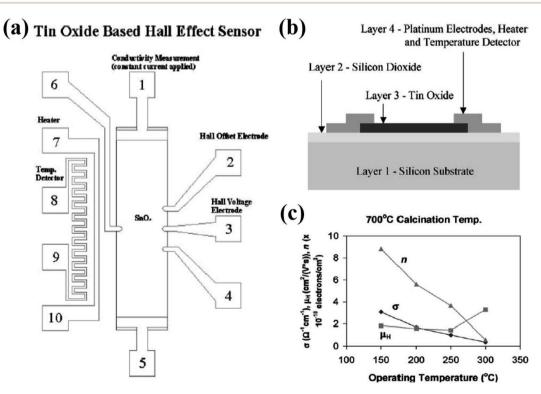
Fig. 4 (a) Tin-oxide based Hall effect sensor. (b) Cross-sectional view of the tin-oxide based Hall effect sensor. (c) Tin oxide thin film conductivity  $(\sigma)$ , electron density  $(\eta)$ , and Hall mobility  $(\mu_H)$  in air vs. operating temperature for sensor calcined at 700 °C. Reprinted with permission from ref. 44. Copyright (2001) Elsevier.
