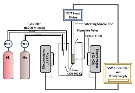
Fig. 2 Schematic of the experimental set-up of the magnetization change-based magnetic gas sensor.
