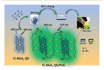
Fig. 1 Schematic illustration of the preparation of the FL-MoS<sub>2</sub>/PVA composites through hydrogen bonding between the FL-MoS<sub>2</sub> QDs and PVA.
