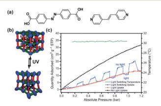
Fig. 8 (a) Structure of the stilbene bispyridyl pillar and azobenzene dicarboxylic acid used as linkers. (b) Depiction of the active framework. (c) Changes in the CO<sub>2</sub> adsorption isotherm of the material (black line, pristine), during in situ irradiation (red line) and upon a modulated exposure to light (blue line), temperature of the sample (green line). Reprinted with permission from ref. 106. Copyright 2013 Wiley-VHC.
