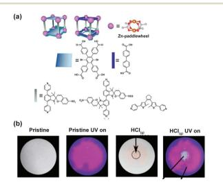
Fig. 25 (a) Structure of the linkers, nodes and schematic depiction of the frameworks structure used in the study. (b) Optical micrographs of the MOF bearing spiropyran pillars pristine material (left panel) and material subjected to HCl vapour at the point indicated by the black arrow (right panel). Adapted with permission from ref. 150. Copyright 2018 American Chemical Society.
