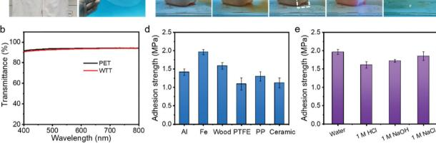
Fig. 4 (a) Photographs of the waterproof transparent tape with a size of  $20 \times 20$  cm. (b) Transmittance of PET and waterproof transparent tape in the visible wavelength range. (c) Photographs showing the ability of the waterproof transparent tape to repair the hole in a bucket in an aquatic environment. (d) Underwater adhesion strength of the waterproof transparent tape for different materials. (e) Adhesion strength of the waterproof transparent tape with Fe in different environments.
