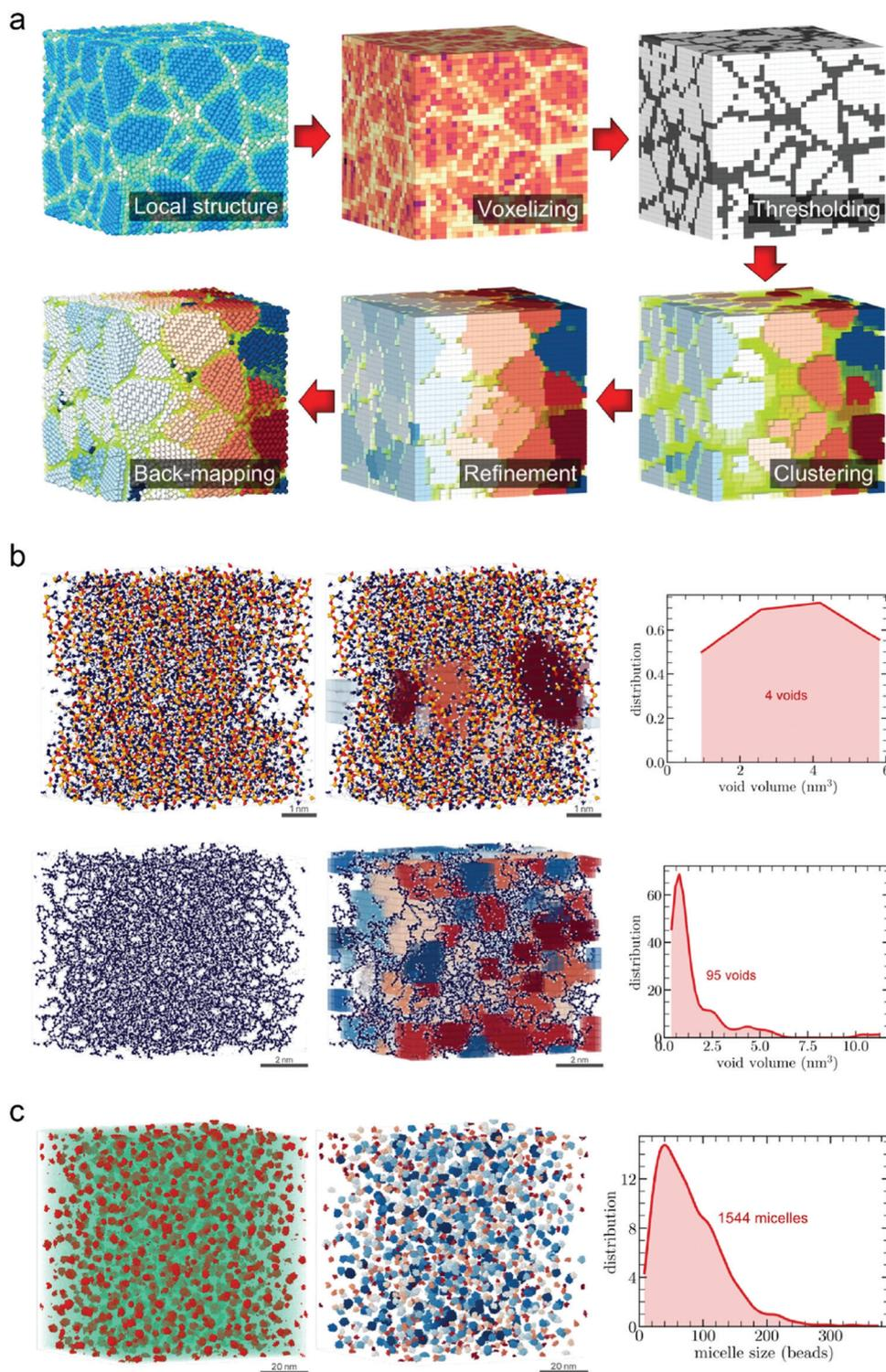
**Fig. 9** An unsupervised approach for the identification and characterization of microstructures in 3-D samples of various material systems. (a) A workflow for autonomous microstructural characterization of 3-D polycrystalline solids. (b and c) Results of the ML-based microstructural analysis method on the analysis of (b) voids in porous materials and (c) micellar distribution in complex solutions (Licensed under CC-BY).<sup>176</sup>
