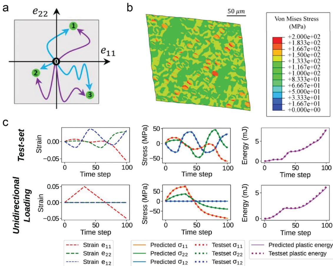
Fig. 5 Learning history-dependent plasticity using recurrent neural networks. (a) Schematic of sampling temporally deformation paths. (b) A deformed heterogeneous representative volume element (RVE) with distributed circular fillers in the generated database. (c) Comparison of the results predicted by recurrent neural networks and calculated from FEM analyses for two different RVEs under different loading conditions (Licensed under CC-BY).<sup>142</sup>
