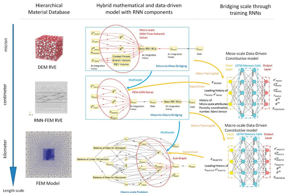
Fig. 8 A multi-scale multi-physics framework for poromechanics problems driven by directed graph representation and recurrent neural networks (Reproduced with permission.<sup>173</sup> Copyright 2018 Elsevier).
