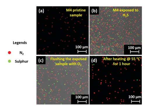
Fig. 6 Surface optical characterization of the M4 material. Energy-dispersive X-ray spectroscopy (EDX) map of (a) a pristine M4 thin film sample, (b) a  $H_2S$ -exposed M4 sample, (c) a  $H_2S$ -exposed M4 sample flushed with  $O_2$  gas, and (d) the complete removal of absorbed  $H_2S$  gas molecules from an M4 sample after heating at 55 °C for 1 hour. Red and green dots represent the presence of  $N_2$  and sulfur elements on the surface of the M4 thin film.
