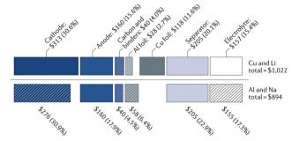
Fig. 1 A cost comparison between lithium-ion and batteries. 13 Copyright 2001, Springer Nature.
