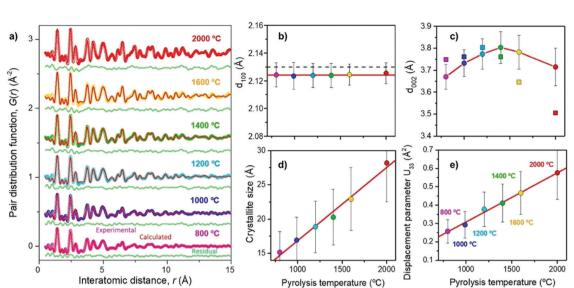
Fig. 20 (a) Experimental (coloured) and calculated using the pairs distribution function method (red), (b)  $d_{100}$  spacing, (c)  $d_{002}$  spacing, (d) crystallite size, and (e) out-of-place displacement parameter of d-spacing of olive pit derived HC samples prepared at temperatures ranging from 800 to 2000 °C. Copyright 2019, American Chemical Society.
