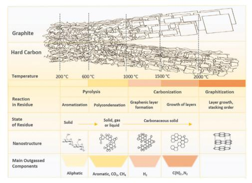
Fig. 13 A schematic illustration representing the changes in chemical and structural characteristics of HC in response to pyrolysis.<sup>86</sup> Copyright 2019, Elsevier
