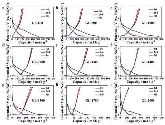
Fig. 27 GCD profiles of HC samples pyrolysed at (a) 600, (b) 800, (c) 1000, (d) 1200, (e) 1300 and (f) 1400 °C, (g) 1500, (h) 1700 and (i) 2000 °C. Copyright 2019, Wiley.
