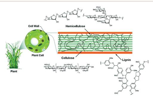
Fig. 12 Lignocellulose composition of plant biomass and the chemical structure of each subunit (cellulose, hemicellulose and lignin).<sup>81</sup> Copyright 2020, Springer Nature.
