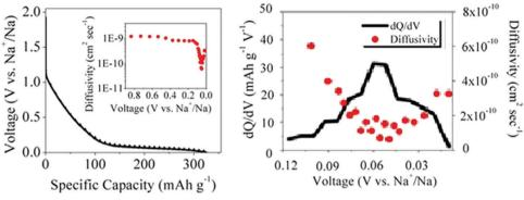
Fig. 9 (a) GITT discharge profiles and sodium-ion diffusivity (inset), and (b) variation of dQ/dV and sodium-ion diffusivity as a function of voltage for a HC.<sup>56</sup> Copyright 2015, American Chemical Society.
