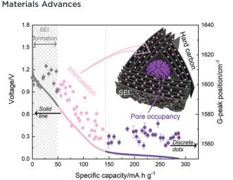
Fig. 6 The GCD profile (solid line) and relative G-band peak position (discrete dots) during first discharge cycle: grey (line and dots) refers to the formation of solid electrolyte interface (SEI), pink (line and dots) refers to intercalation of sodium-ions between graphene layers, and purple (line and dots) refers to filling of sodium ions in pores. 46 Copyright 2020, American Chemical Society
