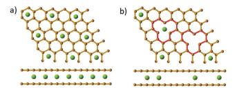
Fig. 22 Illustration of Na-ion storage formulation between (a) pristine graphite and (b) vacancy-defective graphite. 32 Copyright 2018, Wiley.
