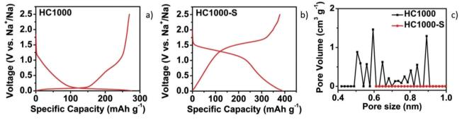
Fig. 8 GCD curves of HC samples without (a) and with sulphur filling in pores (b). (c) DFT pore size distribution curves of samples before (HC1000) and after sulphur filling (HC1000-S).<sup>52</sup> Copyright 2018, Wiley.
