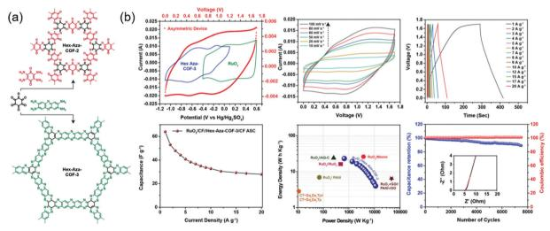
Fig. 6 Electrochemical performance of COF based asymmetric capacitor. (a) Synthesis and design of Hex-Aza-COFs. (b) Electrochemical performance of RuO<sub>2</sub>/Hex-Aza-COF-3 in an asymmetric device. Reproduced with permission.<sup>76</sup> Copyright 2020, Wiley VCH
