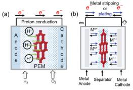
Fig. 18 Representation of working principles in (a) COFs proton conductor in polymer electrolyte membrane fuel cells (PEMFCs). (b) Metal stripping and plating through a COF based soli-state electrolyte acting as ion conductor.
