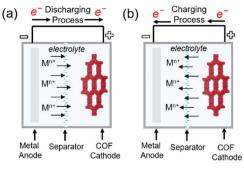
Fig. 8 Representation of working principles in alkali metal-COF hybrid batteries. (a) Discharging process (b) charging process in metal-COF batteries.
