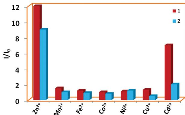
Fig. 11 Bar plot for relative emission intensities of **1** and **2** in the presence of one and two equivalents of metal ions in DMF : H<sub>2</sub>O (1 : 1), respectively.
