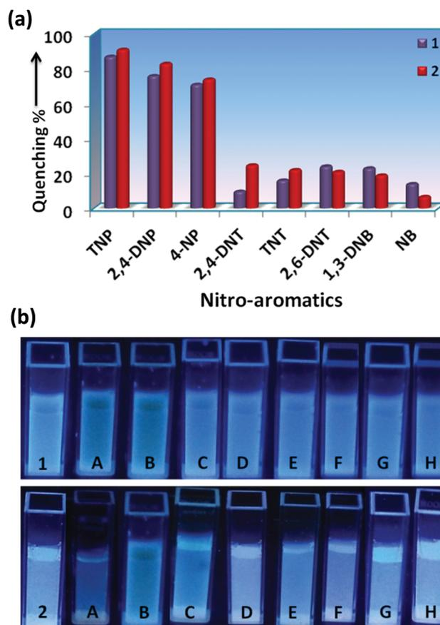
Fig. 3 (a) Fluorescence quenching (%) of **1** and **2** dispersed in water (1 mg, 2 mL) by different NACs (200 μL, 1 mM). (b) Cuvette photographs of **1** and **2** before and after the addition of 200 μL of different analytes upon UV-light illumination at  $\lambda = 365$  nm, where, A: TNP; B: 2,4-DNP; C: 4-NP; D: 2,4-DNT; E: TNT; F: 2,6-DNT; G: 1,3-DNB; H: NB.
