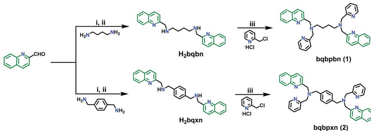
Scheme 2 Synthesis of **1** and **2**: (i) CH<sub>3</sub>OH, stir, 30 °C, 6 h; (ii) NaBH<sub>4</sub> (3 equiv.)/0 °C, stir, 30 °C, 24 h; (iii) H<sub>2</sub>O, NaOH (4 equiv.), pH = 12, stir, 30 °C, 24 h.
