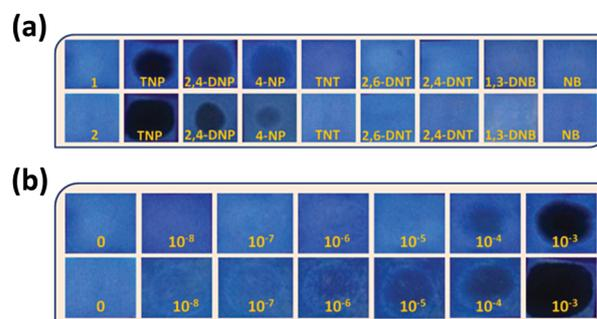
Fig. 10 (a) Paper strips encrusted with **1** (top) and **2** (bottom) and their respective visualisation in the presence of different NACs under UV light ( $\lambda = 365 \text{ nm}$ ). (b) Photographs of paper strips coated with **1** (top) and **2** (bottom) with increasing concentration of TNP ( $10^{-8}$  to  $10^{-3}$  M).
