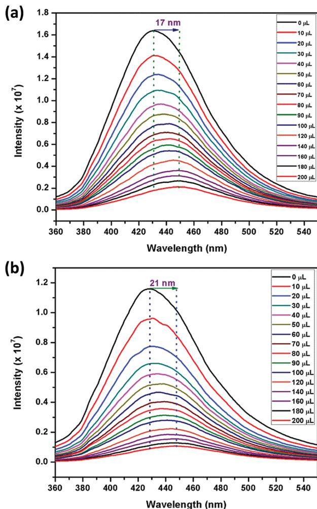
Fig. 2 Effect on the emission spectra of (a) **1** and (b) **2** dispersed in Milli-Q water (1 mg, 2 mL) upon incremental addition of TNP (1 mM) ( $\lambda_{\text{exc}} = 340$  nm).
