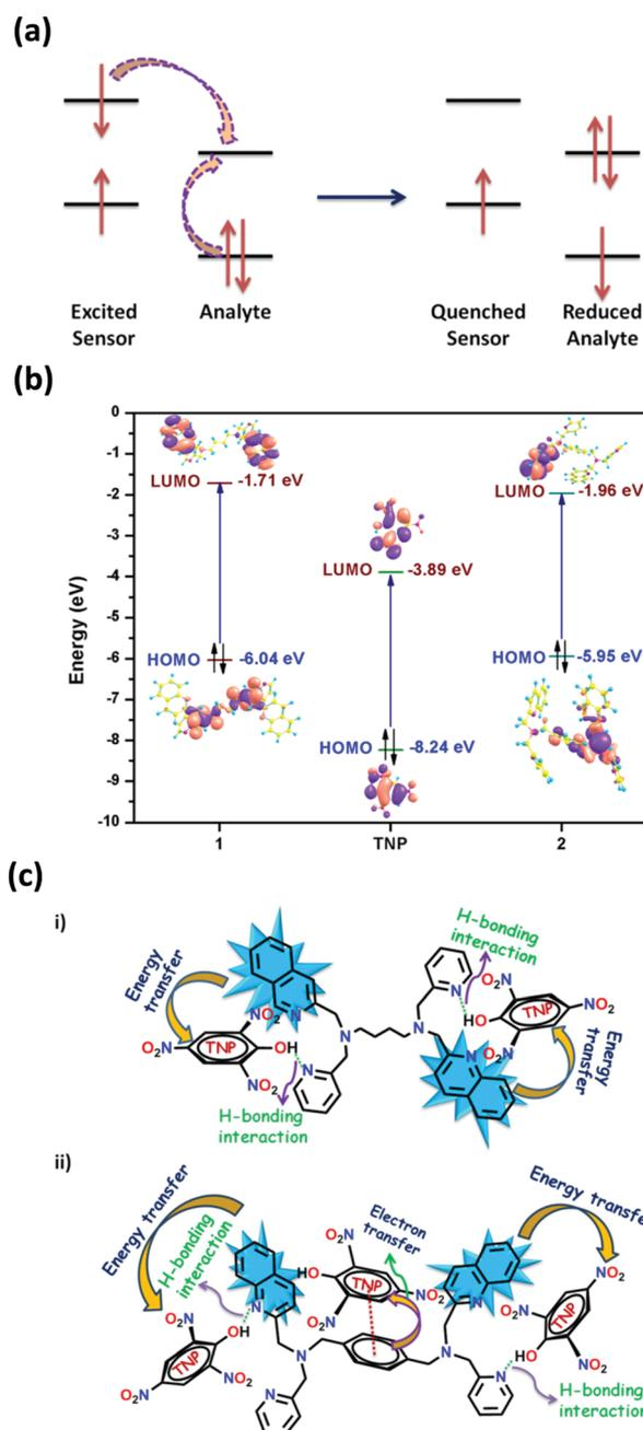
Fig. 6 (a) Schematic illustration of the quenching mechanism via photo-induced electron transfer. (b) Calculated energy diagram with the HOMO–LUMO energies of **1**, **2** and TNP. (c) Possible mechanism of TNP sensing in (i) **1** and (ii) **2**.
