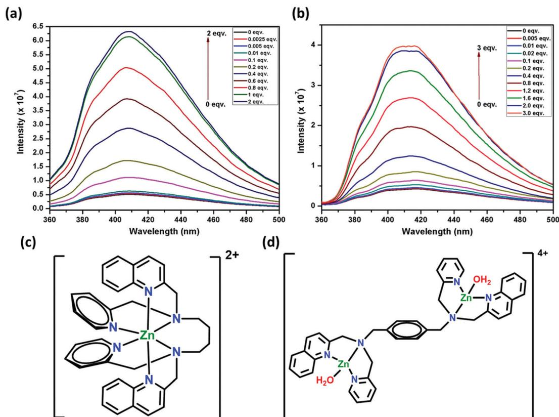
Fig. 12 Emission spectra of (a) **1** and (b) **2** (32 μM) in DMF : H<sub>2</sub>O (1 : 1) with an increase in concentration of Zn<sup>2+</sup> ranging from 0 to 64 μM and 0 to 96 μM, respectively ( $\lambda_{\text{exc}} = 340$  nm). Schematic representation of 1 : 1 and 1 : 2 complex formation in the presence of one and two equivalents of Zn<sup>2+</sup> ion for **1** (c) and **2** (d), respectively.
