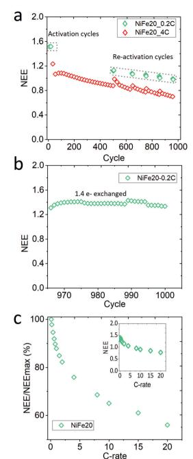
Fig. 5 Characterisation of NiFe20 stability: (a) long-term stability test, (b) after the long-term stability test the electrode is repressed and the capacity of NiFe20 goes back to 1.4e exchanged, and (c) high rate performance of the repressed electrode after the long-term stability test represented by NEE normalised by NEE at 0.1C.
