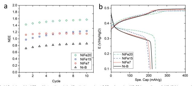
Fig. 3 (a) Evolution of the NEE per Ni atom through the 10 activation cycles at 0.2C performed on NiFe20 (green diamond), NiFe15 (blue square), and NiFe7 (red circles), compared to  $\beta$ -Ni(OH)<sub>2</sub> Ni-B (black triangle). (b) Charge and discharge curves as a function of the specific capacity (mA h g<sup>-1</sup> of compound) for the 10th activation cycle C-rate = 0.2C
