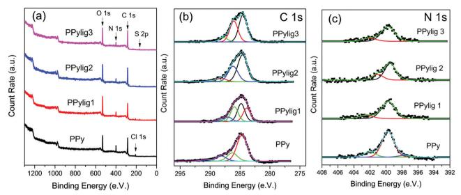
Fig. 3 (a) XPS survey spectra of PPy and PPy with different lignin concentrations, (b) C 1s detailed spectra of PPy and the PPy/lignin composites and (c) N 1s spectra of PPy and the PPy/lignin composites.
