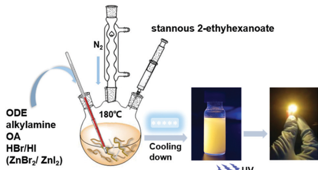
Scheme 1 Schematic diagram of the synthesis of the 2D (\text{RNH}_3)_2\text{SnX}_4 perovskites by a hot-injection method.
