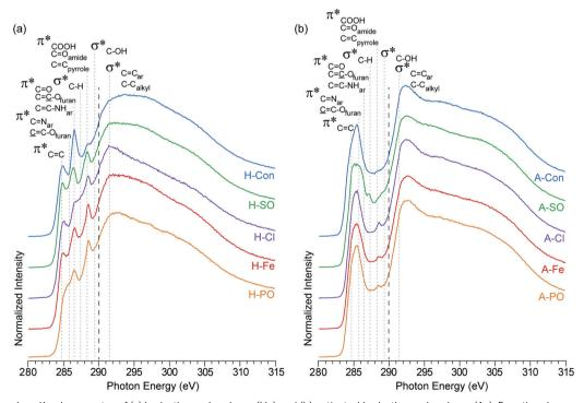
Fig. 3 NEXAFS carbon K-edge spectra of (a) hydrothermal carbons (H-) and (b) activated hydrothermal carbons (A-). Functional group locations for the main C1s  $\to \pi^*$  and C1s  $\to \sigma^*$  are added for reference and based on previous NEXAFS work on hydrothermal carbons. The long dashed lines represent the position of the arctangent step function at 290.0 eV.
