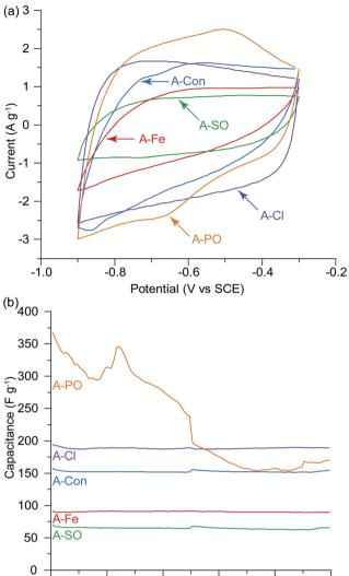
Fig. 5 (a) Cyclic voltammograms at the 500th cycle before the SPECS experiment, (b) capacitance per cycle over 1000 cycles,  $10 \text{ mV s}^{-1}$  in 1 M KOH. The SPECS experiment was conducted at the 500th cycle, hence the slight discontinuity in the capacitance at cycle 500. Decomposition of the electrode/electrolyte was observed for A-PO.
