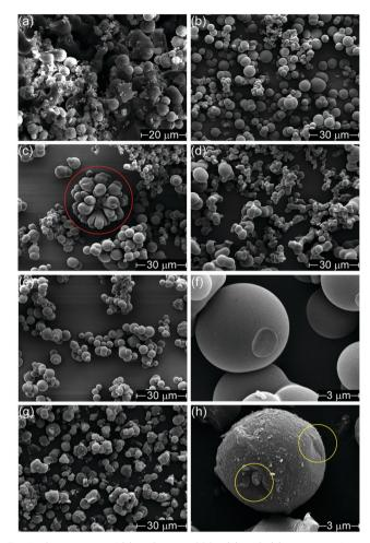
Fig. 1 SEM images of (a) H-Con at  $4000 \times$  (b) H-Cl (c) H-Fe with flower shape outlined in red, (d) H-PO, (e) H-SO, (f) H-SO at 24 000×, (g) A-SO and, (h) A-SO at 24000× with removed sections outlined in yellow. Images were taken at 3000× magnification, unless otherwise specified.
