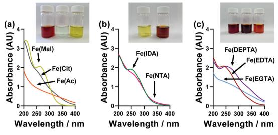
Fig. 6 UV-Vis spectroscopic absorption spectra of the semi-optimised Fe(ligand) systems, using only 2.5 mM Fe(III) and a 1 mm pathlength. The data for Fe(II) and Fe(II/III) solutions can be found in Fig. S6.† The inset photographs in each figure are for the 100 mM solutions used in the thermogalvanic measurements, from left to right; Fe(Ac), Fe(Mal), Fe(Cit), Fe(IDA), Fe(EDTA), Fe(EDTA) and Fe(DEPTA).
