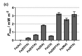
Fig. 3 Bar charts showing (a) the observed Seebeck coefficient ( $S_{\rm e}$ ), (b) the short-circuit current density ( $j_{\rm SC}$ ) and (c) the maximum power density ( $P_{\rm max}$ ) for the semi-optimised Fe(ligand) systems, visually displaying the values in Table 1.
