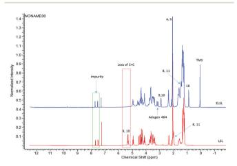
**Fig. 2** Proton NMR spectra of commercial lactonic sophorolipid (LSL, bottom) and epoxidised lactonic sophorolipid product (ELSL, top), showing functional changes upon a successful transformation from LSL to ELSL. AV 700 MHz Bruker spectrometer, CDCl<sub>3</sub> solvent.
