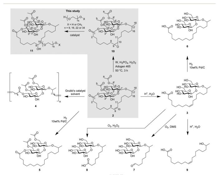
**Scheme 1** Modifications on the double bond of sophorolipid's fatty acid<sup>24,26,28–30</sup> and synthesis of lactonic sophorolipid epoxide (ELSL) from lactonic sophorolipids (LSL) and subsequent modification to PEGylated surfactants (this study).
