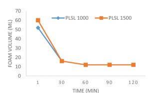
Fig. 8 Foam stability of surfactants over time at solution concentration of 0.25% at 11 000 rpm.
