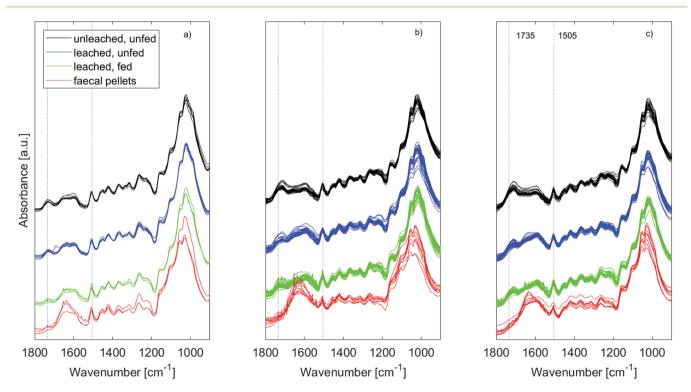
Fig. 5 ATR-IR spectra of wood used in feeding trial II and of faecal pellets from the same feeding trial. Untreated wood shown in (a), treatment 1 in (b) and treatment 2 in (c). As expected, a relative decrease in cellulose content and a relative increase in lignin content is seen after digestion.
