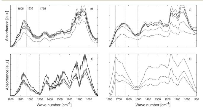
Fig. 6 AFM-IR spectra of gribble faecal pellets (feeding trial I, treatment 2) obtained after 7 (a) and 28 days (b) of feeding on untreated wood, and 7 (c) and 28 days (d) of feeding on furfurylated wood.
