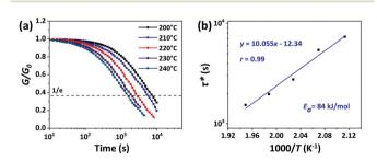
Fig. 3 (a) The normalized stress relaxation of CPA/ESO networks (R = 1.25, TBD 5 mol%) at 200, 210, 220, 230, and 240 °C, respectively. (b) Fitting of the experimental values of relaxation times ( $\tau^*$ ) derived from (a) to an Arrhenius-type equation.
