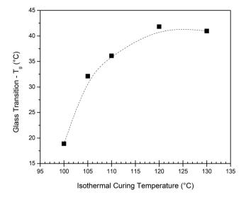
Fig. 3 Obtained  $T_q$  of samples cured for 2 h at different isothermal curing temperatures. The  $T_{
