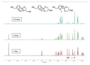
Fig. 2 Crude <sup>1</sup>H NMR spectra of the reaction between HMF and glycerol after 1, 2, and 2.5 days at 40 °C and 20 mbar (on average). Singlet peaks between 6.0 and 5.4 ppm correspond to the C-H peaks of the four isomers. From left to right: Dioxolanes, cis-dioxane, trans-dioxane. The decrease of the HMF peaks during the reaction is also visible, e.g. aldehyde peak at 9.55 ppm.
