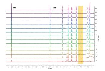
Fig. 5 <sup>1</sup>H NMR degradation study of 3-10% over time in 0.1 M HCl in acetone showing the disappearance of the acetal peak at 5.55 ppm over time and appearance of the HMF aldehyde peak.
