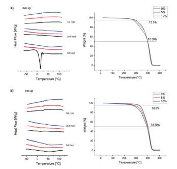
Fig. 4 Thermal properties of PU films. (a) DSC and TGA of type A (4), (b) DSC and TGA traces of type B (5).
