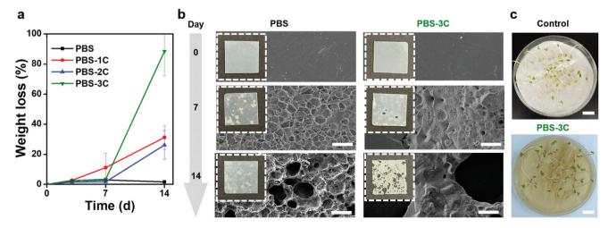
Fig. 5 (a) Bio-decomposition (weight loss) of the PBS series in composting soil. (b) Optical and SEM images of film surfaces before and after biodecomposition (film sizes: 10 x 10 mm, scale bar: 10 µm). (c) Optical images of germinated lettuce seeds after the bio-decomposition experiments of PBS-3C and the negative control (scale bar: 1 cm).
