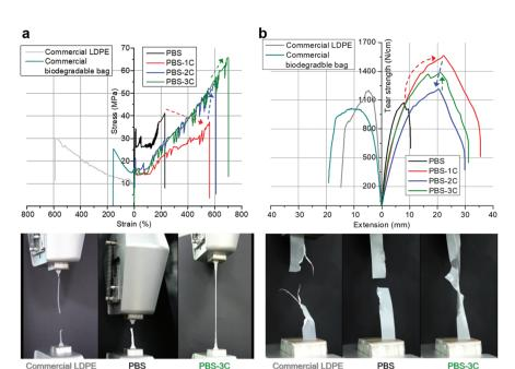
Fig. 2 (a) Tensile stress-strain and (b) tear-strength-extension curves of prepared films and commercial reference films. Bottom: photographic images acquired during mechanical testing.
