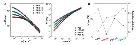
Fig. 4 Rheological responses of the PBS series at 140 °C. (a) Complex viscosities ( $\eta^*$ ), (b) storage moduli (G), and (c) variations in G at 0.05 rad s<sup>-1</sup>  $(G'_{0.05})$  and Cole-Cole plot slopes.
