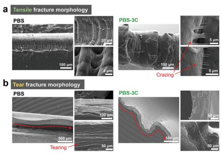
Fig. 3 SEM images of the fractured surfaces of (a) tensile- and (b) tear-tested PBS and PBS-3C specimens.
