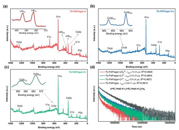
Fig. 4 XPS spectra of the Tb-FAP/agar after treatment with (a) UO<sub>2</sub><sup>2+</sup>, (b) Cu<sup>2+</sup>, and (c) Cr<sup>3+</sup> accompanied with the insets showing the detailed XPS spectra of U 4f, Cu 2p, and Cr 2p, respectively. (d) The luminescence lifetime spectra of the Tb-FAP/agar sample recorded in the presence and absence of Cu<sup>2+</sup>, Cr<sup>3+</sup>, and UO<sub>2</sub><sup>2+</sup> ions ( $\lambda_{ex}$  = 377 nm and  $\lambda_{em}$  = 543 nm).
