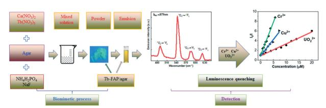
Scheme 1 Schematic for the biomimetic process of the Tb-FAP/agar sample and the subsequent detection of UO22+, Cu2+, and Cr3+ ions in aqueous solution.
