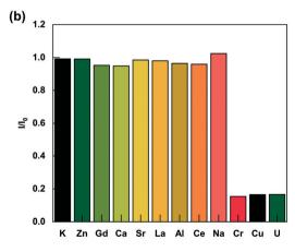
Fig. 2 (a) The emission spectra of the Tb-FAP/agar, Tb-FAP agar free, and Tb-HAP/agar samples. (b) Luminescence intensity of the  $^5D_4 \rightarrow ^7F_5$ transitions (543 nm) of the Tb-FAP/agar (2.5 mL) with different metal ions (10  $\mu$ L, 0.01 M).
