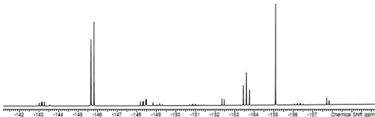
Fig. 7 The  $^{19}\text{F}\{^1\text{H}\}$  NMR spectrum of  $[\text{SnF}_3(\text{dmsO})_3][\text{OTf}]$  (298 K) showing the resonances of the two isomers with  $^{117/119}\text{Sn}$  satellites (the OTf resonance is not shown).
