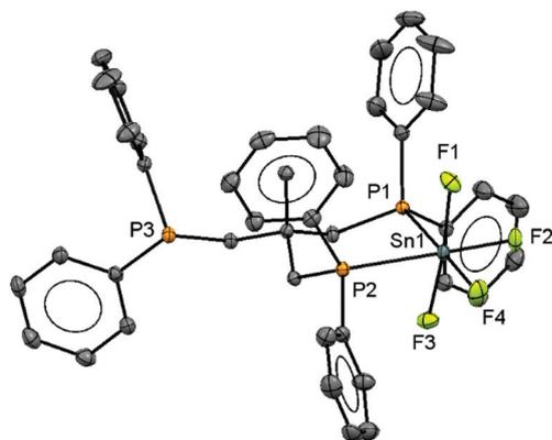
**Fig. 1** Crystal structure of [SnF<sub>4</sub>( $\kappa^2$ -triphos)] showing the atom labelling scheme. The ellipsoids are drawn at the 50% probability level and H atoms are omitted for clarity. Selected bond lengths (Å) and angles (°) are: Sn1–P1 = 2.6302(5), Sn1–P2 = 2.6314(5), Sn1–F1 = 1.9670(12), Sn1–F2 = 1.9488(12), Sn1–F3 = 1.9791(12), Sn1–F4 = 1.9307(12), P1–Sn1–P2 = 91.245(14), P1–Sn1–F4 = 172.46(5), P2–Sn1–F2 = 174.74(4), F1–Sn1–F3 = 173.44(5).
