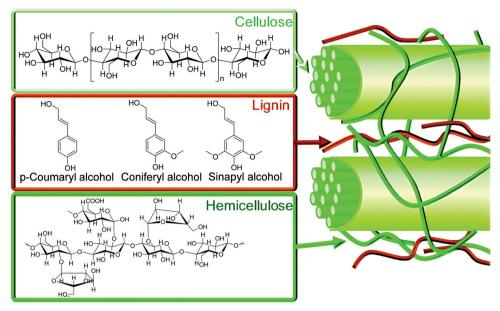
Fig. 1 Structures of cellulose, hemicellulose, and lignin components of lignocellulosic biomass and associated molecular building blocks. Reproduced with permission from ref. 4, Copyright 2012 Royal Society of Chemistry.
