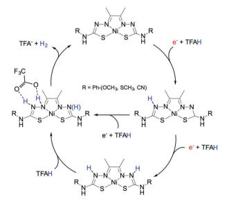
Fig. 18 DFT computed reaction mechanism for hydrogen evolution mediated by a molecular catalyst highlighting the influence of the proton source on the preferable pathway. Adapted with permission from ref. 309. Published by The Royal Society of Chemistry.
