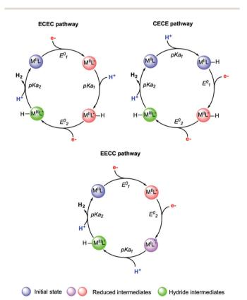
Fig. 14 Selected examples of sequences and putative intermediates considered during hydrogen evolution reaction. Adapted with permission from ref. 291. Copyright 2019 Chem Pub Soc.
