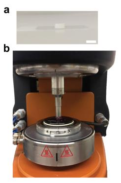
**Fig. 2** Experimental setup. (a) Ionically Ca<sup>2+</sup> cross-linked ADA-GEL hydrogel sample. Scale bar: 10 mm (b) testing setup with sample mounted to the rheometer and surrounded by cell culture medium (DMEM) to avoid dehydration.
