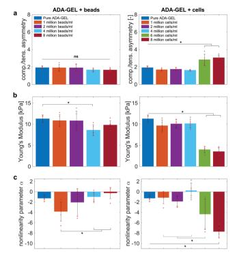
Fig. 9 Average compression—tension asymmetry (a), Young's modulus (b), and non-linearity parameter  $\alpha$  (c) with standard deviations for beadand cell-laden ADA-GEL samples with different filler densities. Asterisks denote statistical significance analysed via one-way ANOVA followed by Tukey–Kramer tests for multiple comparisons (\*p < 0.05).
