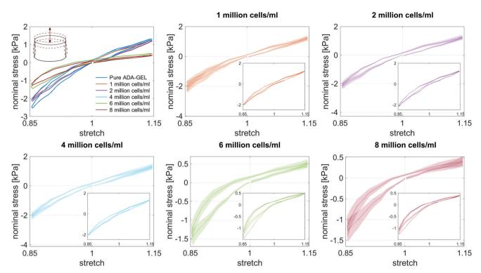
Fig. 6 Response of cell-laden ADA-GEL samples with different cell densities during cyclic compression—tension experiments up to a maximum strain of 15%. The large graphs show the average conditioned response during the third loading cycle with standard deviations, while the small insertions illustrate the conditioning behavior during the whole set of three loading cycles.
