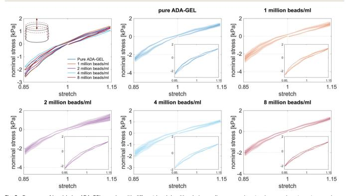
Fig. 5 Response of bead-laden ADA-GEL samples with different bead densities during cyclic compression—tension experiments up to a maximum strain of 15%. The large graphs show the average conditioned response during the third loading cycle with standard deviations, while the small insertions illustrate the conditioning behavior during the whole set of three loading cycles.
