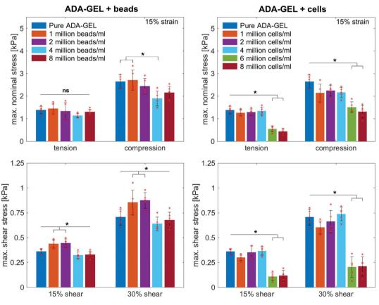
Fig. 8 Average maximum stresses with standard deviations during cyclic compression, tension, and torsional shear experiments for bead- and cell-laden ADA-GEL samples with different filler densities. Asterisks denote statistical significance analysed via one-way ANOVA followed by Tukey–Kramer tests for multiple comparisons (\*p < 0.05).
