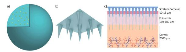
Fig. 3 3D models of a nanoparticle with drug cargo (a) and a microneedle array (b) and a diagram showing the application of the microneedle array through skin (c).
