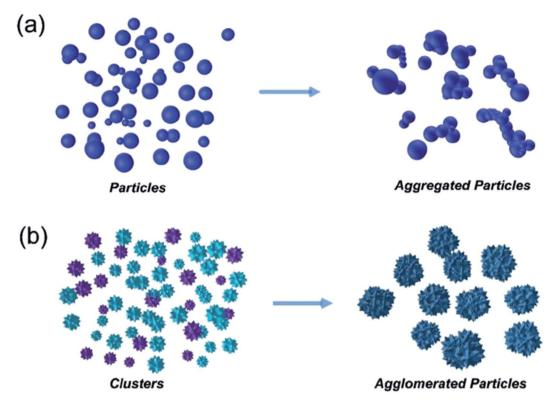
Fig. 2 Diagram showing the mechanism difference between aggregation (a) and agglomeration (b).<sup>48</sup>
