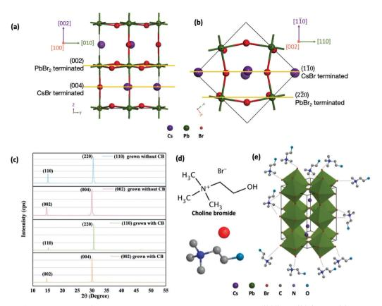
Fig. 2 (a) Side view of the orthorhombic CsPbBr<sub>3</sub> unit cell structure. The yellow lines indicate (002) and (004) plane. (b) Top view of the unit cell structure. The yellow lines indicate  $(1\bar{1}0)$  and  $(2\bar{2}0)$  plane. (c) XRD pattern of CsPbBr<sub>3</sub> single crystal grown with and without CB. (d) Molecular structure of choline bromide (CB). (e) Schematic illustration of CB assisted CsPbBr<sub>3</sub> single crystal growth.
