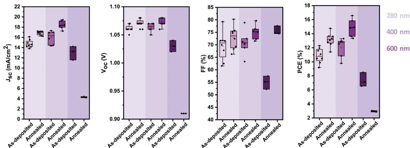
Fig. 6 Photovoltaic performance parameters ( $V_{OC}$ ,  $J_{SC}$ , FF and PCE) of stoichiometric photovoltaic devices with active layers of 280 nm, 400 nm and 600 nm before and after annealing at 100 °C.
