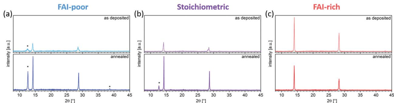
Fig. 4 X-ray diffraction patterns of (a) FAI-poor, (b) stoichiometric, and (c) FAI-rich perovskite samples prepared on glass substrates before and after annealing at 100 °C. Reflections originating from  $\text{PbI}_2$  are marked with a \*.
