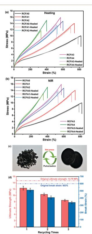
Fig. 7 (a) Typical stress-strain curves of RCFA healed at 140  $^{\circ}$ C for 30 min. (b) Typical stress-strain curves of RCFA healed under NIR irradiation for 20 min. (c) Optical images of reprocessing ability of RCFA2. (d) Mechanical property recovery of recycled RCFA2.
