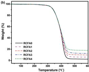
Fig. 4 (a) DSC curves of RCFA with different modified MWCNT contents. (b) TGA curves of RCFA with different modified MWCNT contents.
