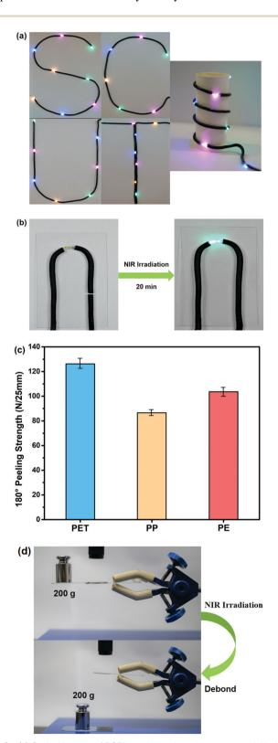
Fig. 9 (a) Optical images of RCFA used as an interconnect material in LED arrays. (b) Fast self-healing of RCFA used as an interconnect material in supporting LEDs. (c) 180° peeling strength of RCFA on various substrates. (d) Optical images of the joint debonded by NIR irradiation.
