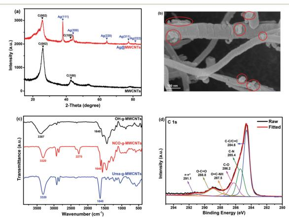
Fig. 2 (a) XRD patterns of MWCNTs and Ag@MWCNTs. (b) SEM images of Ag@MWCNTs. (c) FTIR spectra of OH-g-MWCNTs, NCO-g-MWCNTs and urea-g-MWCNTs. (d) XPS elemental survey data of urea-g-MWCNTs.
