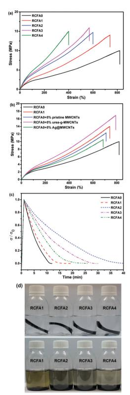
Fig. 5 (a) Stress-strain curves of RCFA with different modified MWCNT contents. (b) Stress-strain curves of RCFA with different types of modified MWCNTs. (c) Stress relaxation curves of RCFA with different modified MWCNT contents at 140 °C. (d) Solubility of RCFA in DMF at room temperature for 5 d and 140 °C for 2 h.
