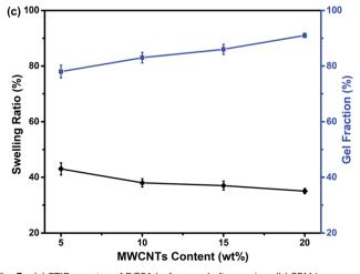
Fig. 3 (a) FTIR spectra of RCFA before and after curing. (b) SEM images of RCFA with different contents of modified MWCNTs. (c) Swelling ratio and gel fraction of RCFA with different modified MWCNT content.
