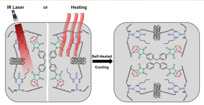
Fig. 6 Illustration of self-healing process of RCFA.
