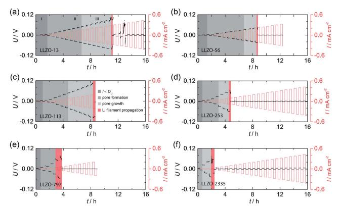
Fig. 2 Galvanostatic cycling, that is, striping and plating experiments, of the symmetric Li|LLZO|Li cells studied in Fig. 1; measurements were carried out at room temperature (20 °C). U: voltage, I: current density. See text for further explanation.
