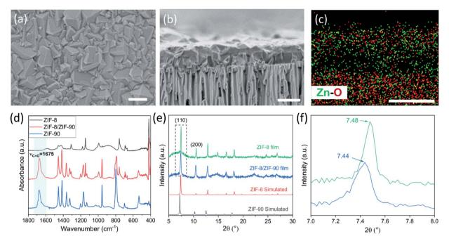
Fig. 6 SEM images of ZIF-8/ZIF-90 film: (a) top view, (b) cross-sectional view and (c) the corresponding elemental mapping. (d) FTIR plots of ZIF-8 film, ZIF-90 powder, and hybrid ZIF-8/ZIF-90 films. (e) XRD of ZIF-8 and hybrid ZIF-8/ZIF-90 films. (f) The enlarged XRD pattern showing the minor shift and broadening of the (110) peak in (e). All scale bars correspond to 1  $\mu$ m.
