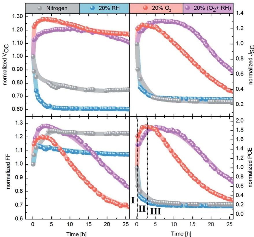
Fig. 2 Evolution of photovoltaic parameters under different atmospheres. From left to right, the panels show the normalized  $V_{oc}$ ,  $J_{sc}$ , FF and PCE. The lines behind the data points are meant as a guide for the eye. In the PCE panel, the three phases of degradation under oxygen (I, II, and III) are defined. The first data point of each curve is always measured in nitrogen only. The gas flow is started after the first measurement.
