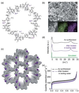
Fig. 1 (a) Chemical structure, (b) SEM and EDS mapping (for S and Zn) images, (c) structural model  $(Zn^{2+}$ : purple, TpPa-SO<sub>3</sub><sup>-</sup>: grey), (d) XRD patterns and (e) N<sub>2</sub> gas isotherms of TpPa-SO<sub>3</sub>Zn<sub>0.5</sub>.
