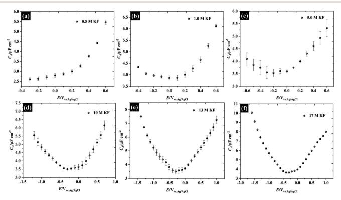
Fig. 2 Capacitance–potential (C-E) curves of highly ordered pyrolytic graphite in (a) 0.5 M, (b) 1.0 M, (c) 5.0 M, (d) 10 M, (e) 13 M, and (f) 17 M potassium fluoride (water-in-KF salt).
