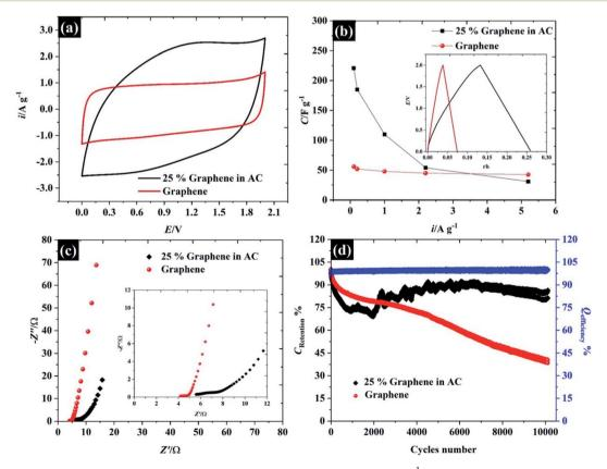
Fig. 9 Performance of supercapacitor devices using 17 M KF electrolyte. (a) CV at 75 mV s<sup>-1</sup>, (b) capacitance and charge/discharge profile at 2.2 A  $g^{-1}$ , (c) Nyquist plot, and (d) cyclic stability at 1.0 A  $g^{-1}$  over 10 000 cycles.
