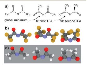
Fig. 10 (a) Schematic representation of the conformational changes in  $[N(TFA)_2]^-$ , (b) the optimised minimum geometries of this anion, (c) the corresponding structures for the non-fluorinated analogue [N(Ac)<sub>2</sub>]<sup>-</sup>.
