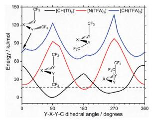
Fig. 11 Slices of the PES of  $[CH(Tf)_2]^-$ ,  $[N(TFA)_2]^-$ , and  $[CH(TFA)_2]^-$ . One of the two S–X–S–C dihedral angles is kept at 90°. The global minimum of the whole PES is used as the zero value.
