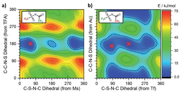
Fig. 13 Potential energy surfaces of the anions (a) [N(Ms)(TFA)]<sup>-</sup> and (b) [N(Tf)(Ac)]<sup>-</sup> in the experimentally investigated ILs. The red crosses correspond to the dihedral angles obtained experimentally from crystal structures of model compounds.
