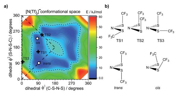
Fig. 5 (a) PES of  $[N(Tf)_2]^-$ , (b) stationary point structures (oxygen atoms not shown). Open circles denote minima, black crosses denote transition states. The dotted line is drawn at 15 kJ  $mol^{-1}$  to facilitate comparison with other surfaces. The lowest energy conformer is taken as the zero reference.
