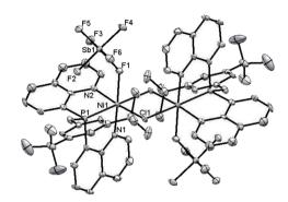
Fig. 1 ORTEP drawing of the X-ray crystal structure of **3b**. Hydrogen atoms and  $C_6H_5F$  are omitted for clarity. Key bond distances (Å): Ni(1)–N(1) = 2.092(6), Ni(1)–N(2) = 2.070(7), Ni(1)–P(1) = 2.347(2), Ni(1)–F(1) = 2.262(4), Sb(1)–F(1) = 1.904(4), Sb(1)–F(2) = 1.873(5), Sb(1)–F(3) = 1.877(5), Sb(1)–F(4) = 1.874(5), Sb(1)–F(5) = 1.867(5), Sb(1)–F(6) = 1.869(5).
