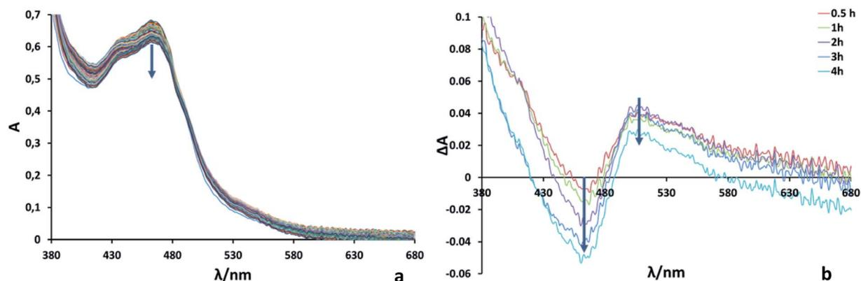
Fig. 3 (a) UV-vis absorption spectra during irradiation of a DMA–TEOA (5 : 1 v/v) solution containing RuRe<sub>2</sub> (50 μM) and BIH (0.1 M) at λ<sub>ex</sub> = 480 nm for 240 min at 1 min intervals. (b) UV-vis differential absorption spectra between before and after irradiation.
