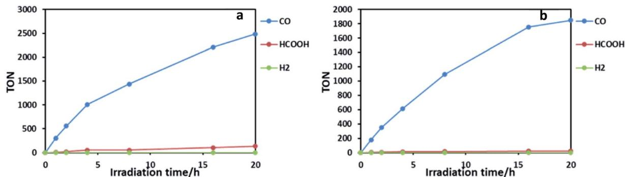
Fig. 2 Photocatalytic formation of CO (blue line), formic acid (red line) and H<sub>2</sub> (green line) as a function of irradiation time using (a) Ru<sub>2</sub>Re and (b) RuRe<sub>2</sub>: CO<sub>2</sub>-saturated DMA–TEOA (5 : 1 v/v, 3 mL) solutions containing Ru<sub>2</sub>Re (25 μM) or RuRe<sub>2</sub> (50 μM) and BIH (0.1 M) irradiated at λ<sub>ex</sub> = 490–615 nm.
