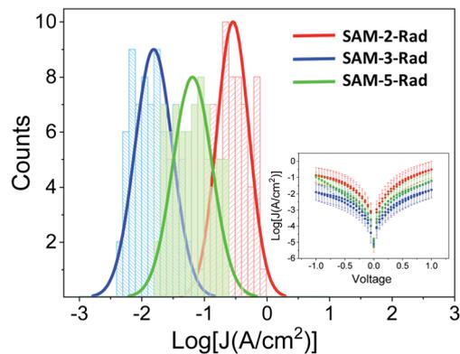
Fig. 6 Histograms and Gaussian fits of  $\log|J|$  at 1 V for junctions Au<sup>TS</sup>/SAM-2,3 and 5-Rad//GaO<sub>x</sub>/EGaIn. Inset: Plots of mean  $\log|J|$  versus  $E(V)$ .
