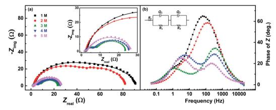
Fig. 9 (a) EIS recorded at EP on carbon-modified GCE with 1600 rpm in equimolar (0.2 M) concentration  $V^{4+}$  and  $V^{5+}$  in  $H_2SO_4$  electrolyte of different concentrations. The corresponding Bode phase plots are shown in (b), along with the equivalent circuit (inset). The symbols and solid lines show the experimental and the fitted data, respectively.
