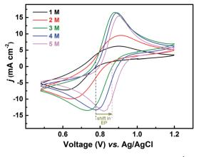
Fig. 8 CVs recorded on carbon-modified GCE at 20 mV s $^{-1}$  scan rate in equimolar (0.2 M) solution of V $^{4+}$  and V $^{5+}$  in H $_2$ SO $_4$  electrolyte of different concentrations. The dotted lines show the shift in EP with supporting electrolyte (H $_2$ SO $_4$ ) concentration.
