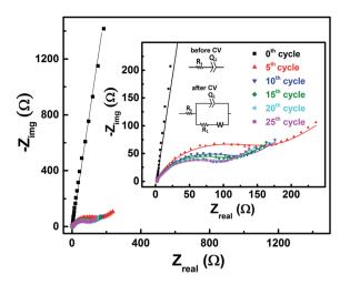
Fig. 6 EIS patterns recorded at OCP on carbon-modified GCE without rotation in 0.2 M  $\rm V^{5+}$  electrolyte after every 5 cycles. The symbols and solid lines show the experimental and the fitted data, respectively. The corresponding EC is shown in the inset.
