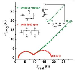
Fig. 2 EIS patterns recorded at EP on carbon-modified GCE without rotation and with 1600 rpm in equimolar (0.2 M) concentration of  $V^{4+}$  and  $V^{5+}$  in 3 M  $\rm H_2SO_4$  electrolyte. The symbols and solid lines show the experimental and the fitted data, respectively. The corresponding ECs are shown in the insets. The expanded view of the  $45^\circ$  line is shown in the inset.
