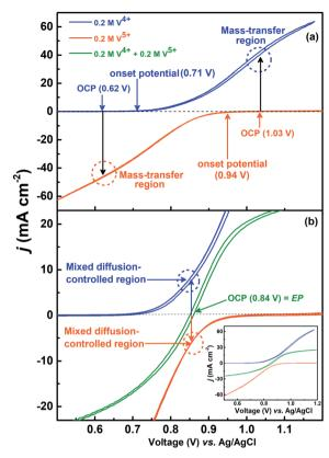
Fig. 4 CVs recorded on carbon-modified GCE at 20 mV s $^{-1}$  scan rate with 1600 rpm in 0.2 M V $^{4+}$  and 0.2 M V $^{5+}$  (a) and equimolar (0.2 M) concentration of V $^{4+}$  and V $^{5+}$  electrolytes (magnified view) (b); the complete CVs of V $^{4+}$  and V $^{5+}$  are included in the inset to (b) for comparison.
