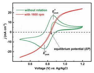
Fig. 1 CVs recorded with carbon-modified GCE without rotation and with 1600 rpm at 20 mV s $^{-1}$  scan rate in equimolar (0.2 M) concentration of V $^{4+}$  and V $^{5+}$  in 3 M H $_2$ SO $_4$  electrolyte.
