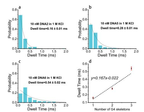
Fig. 5 Nanopore translocation duration of G4 recorded with 100 nM DNA2, DNA5 and DNA6, performed in 1 M KCl, 10 mM Tris, 1 mM EDTA at pH 7.4 under 200 mV bias voltage in an  $\sim$ 4.2 nm nanopore. (a–c) Histograms of dwell time with exponential decay fitting curves; all the data were treated with the same bin size of 0.2 ms. (d) Line fitting graph of dwell time as a function of the number of G4 skeletons.
