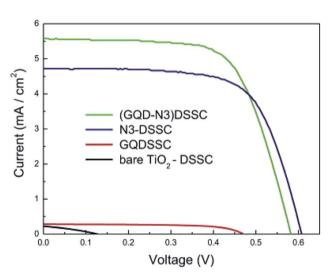
Fig. 22 J-V characteristics curves of DSSCs with bare GQD, N<sub>3</sub>, TIO<sub>2</sub> and combination of GQD and N<sub>3</sub> were taken under 1 sun illumination intensity. Reproduced with permission from ref. 214, copyright 2015, Elsevier.
