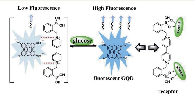
Fig. 10 Sensing mechanism based on BBV receptor and fluorescent GQDs. Reproduced with permission from ref. 116, copyright 2013, The Royal Society of Chemistry.
