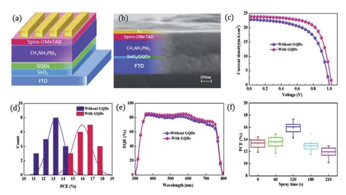
Fig. 19 (a) schematic diagram of perovskite solar cell. (b) Cross sectional SEM image of perovskite structure. (c) J-V curves of the PSC based on  $SnO_2$  with and without GQDs. (d) Statistic histogram of the power conversion efficiency (PCE) (e) external quantum efficiency spectra. (f) PCE tendency with different time period. Reproduced with permission from ref. 211, copyright 2019, Elsevier.
