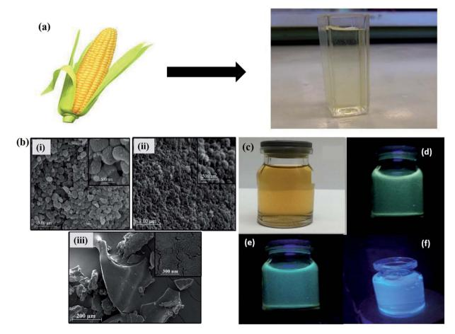
Fig. 8 (a) Schematic diagram of GQDs synthesis through green chemistry (b) SEM images of as-prepared GQDs, TiO2 and GQDs/TiO2 composite, (c) as-synthesized GQDs under normal light and (d-f) UV light. Reproduced with permission from ref. 85, copyright 2017, Elsevier.
