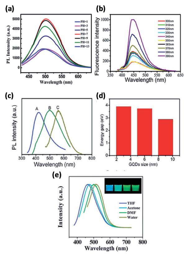
Fig. 9 (a) Fluorescence spectra of GQDs at different pH. Adapted from ref. 110, copyright 2015, PLoS One publication. (b) Different excitation wavelengths. Reproduced with permission from ref. 111, copyright 2018, Elsevier. (c and d) Different size of GQDs and their band gap energy. Adapted from the ref. 83, copyright 2016, American Scientific Publisher. (e) Different solvents. Reproduced with permission from ref. 21, copyright 2011, The Royal Society of Chemistry.
