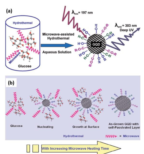
Fig. 5 (a) Schematic diagram of synthesis of GQDs via microwave-assisted hydrothermal (MAH) technique and (b) schematic diagram of mechanism of formation of GQDs with functional groups. Adapted from the ref. 69. Copyright 2012, ACS Publications.
