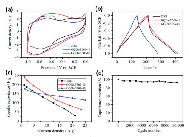
Fig. 18 (a) Cyclic voltammetry curve at a scan rate of  $10 \text{ mV s}^{-1}$  (b) charge/discharge curves at different current densities with different compositions, respectively (c) specific capacitance versus current densities and (d) cycling stability at a current density of 24 A g<sup>-1</sup> for the composite material. Adapted from ref. 183, copyright 2019, MDPI publications.
