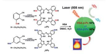
Scheme 1 Schematic illustration of synthesis of HSA-α-Pc and HSA**β-Pc** NPs and their phototherapy effects.
