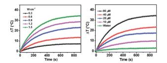
Fig. 3 Photothermal property of HSA-α-Pc NPs in aqueous solution under 808 nm laser irradiation. Left: Light intensity-dependent temperature increase at the concentration of 80 μM (Pc equiv.). Right: Concentration-dependent temperature increase with a 0.9 W cm<sup>-</sup> laser intensity.
